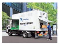
SG Moving pulping vehicle (four-ton truck)
